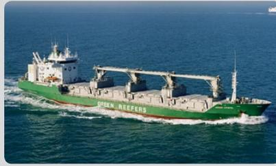
The vessel is fully grating fitted and is built for a high flexibility for shipment of chilled/frozen cargo of both palletized and loose configuration.
